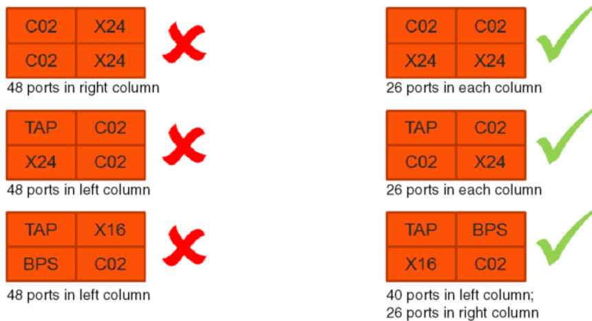
Figure 7 Module Placement of PRT-HC0-CO2, 100G Mode
